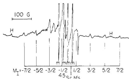
**Figure 1.** ESR spectrum of  $\text{ScCl}_2$  in argon at 14 K. The magnetic field corresponding to  $g_e$  occurs at the center of the methyl quartet denoted by "m". Modulation (100 kHz) was 2 G, and incident microwave power was approximately 1.0 mW for all spectra presented.
