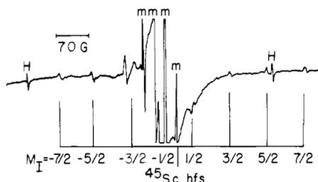
**Figure 2.** ESR spectrum of  $\text{Sc(CN)}_2$  in argon at 14 K. The magnetic field corresponding to  $g_e$  occurs at the center of the methyl quartet denoted by "m".
