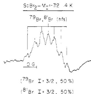
**Figure 3.** Expanded-scale ESR spectrum of the lowest field  $^{45}\text{Sc}$  transition of  $\text{ScBr}_2$  exhibiting Br hfs. The center of the seven-line pattern occurs at 3202 G. Spectrometer frequency is 9526 MHz.
